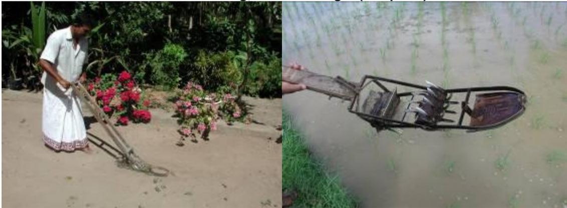
**Figure 17: On left, improved cono weeder designed by H.M. Premaratna, Mellawalana, Sri Lanka, and on right, a model made by local engineer in Madagascar to inter-cultivate two rows at a time, with the option of adjusting the cones for wider or narrower inter-row spacings (N. Uphoff)**
