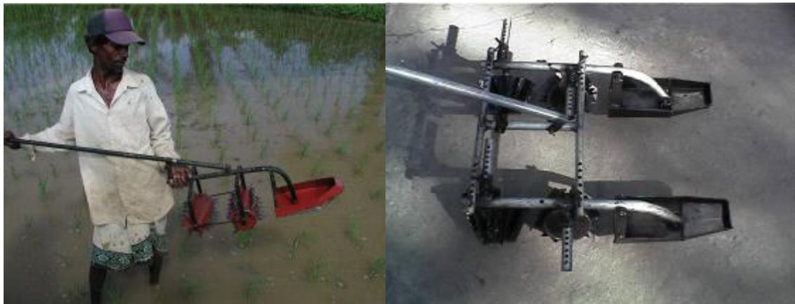
**Figure 18: On left, a weeder designed and built by Nong Sovann, Kandol village, Kampho Speu, Cambodia, from local materials (wooden axle, heavy nails, iron rods) (N. Uphoff); on right, more expensive, motor-powered weeder designed and built by Ariyaratna Subasinghe, System H, Mahaweli project, Sri Lanka (A. Subasinghe)**
