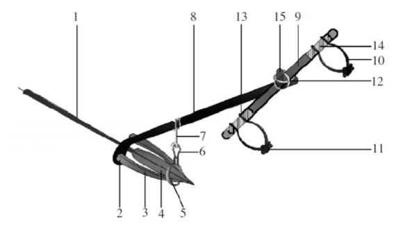
Fig. 2-Three-dimensional sketch of Ethiopian *ard* plough 'Maresha'(1) handle; (2) wooden pin; (3) side-wing; (4) ploughshare; (5) lower metal loop; (6) upper metal loop; (7) leather stripe (8) beam; (9) yoke; (10) neck holder sticks; (11, 12) leather strap or rope; (13) rubber as washer; (14) leather for safety; (15) centering pin. Source: Gebregziabher et al. 2007, p. 30
